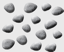
Kugelige Sandkörner aus herkömmlichen Lagerstätten. Spherical sand granules from conventional deposit sites.
